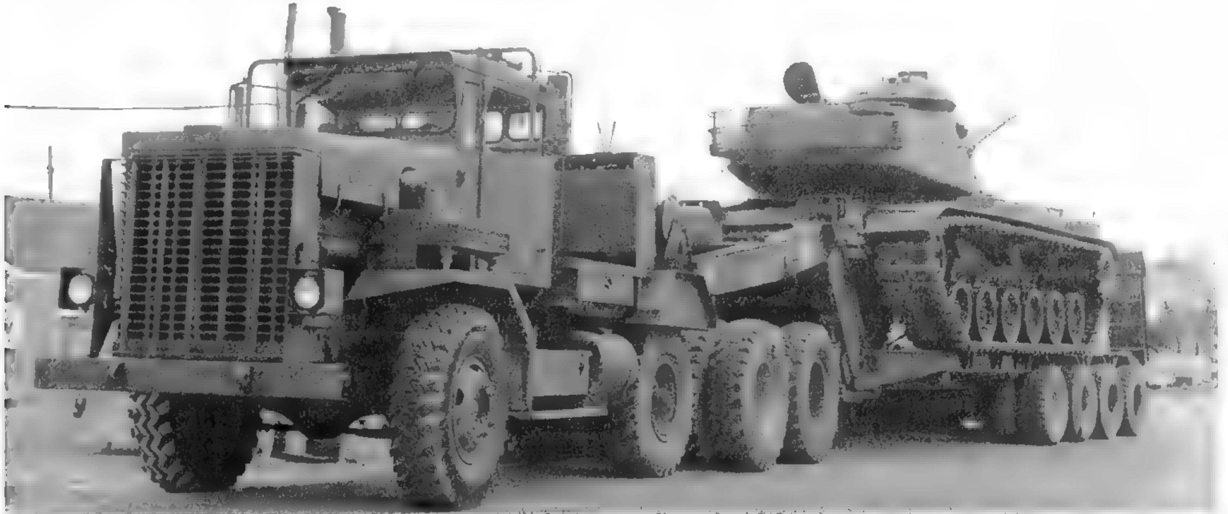
This M911 is shown coupled to its usual trailer, an M747. As expensive as this combination is to operate, it's a bargain compared to road marching a tank. Fully operational tanks were often transported by truck. (U.S. Army photo)
